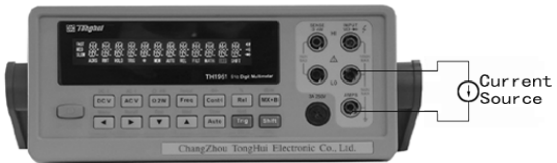
CAUTION: Maximum Input = 3A DC or RMS Figure 3-2 DC and AC Current Measurements
